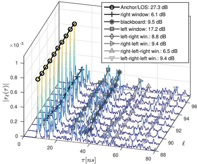
Fig. 5. Impulse response analysis with estimated SINRs of the respective MPCs, BW 2 GHz,  $f_c = 7$  GHz.
