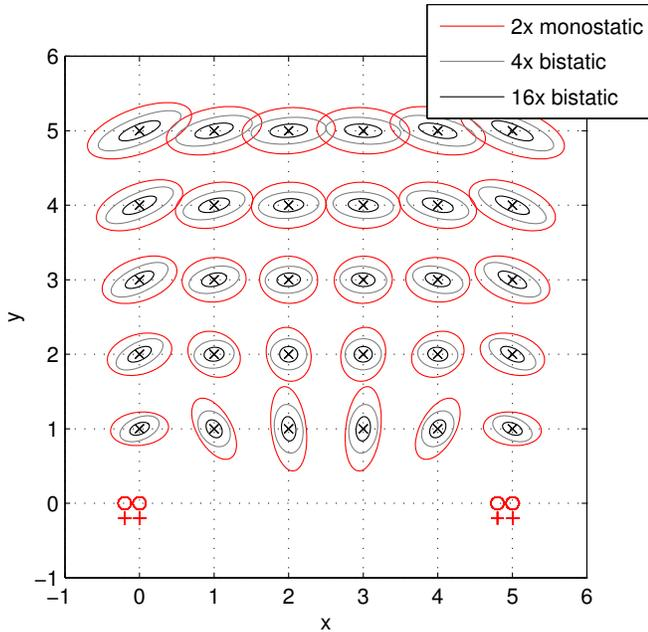
Fig. 3. Position error bound (2-fold STDV ellipses) and MIMO gain on a backscatter channel with a bandwidth of 50 MHz. The different antenna configurations are discussed in the text. Channel Parameters:  $K_{LOS} = 0$  dB,  $\tau_{rms} = 17.5$  ns
