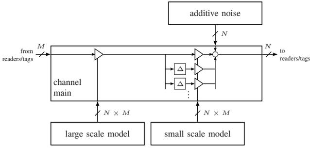
Fig. 4. Channel block diagram. Unlike reader and tag, the channel is XIXO per definition (e.g.  $M$  readers,  $N$  tags). Also the reader to reader channel  $K(\omega, i)$  in Fig. 6 is modeled in this fashion ( $M = N$  readers).
