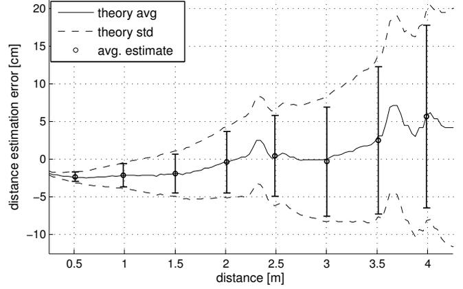
Fig. 9. Example: Two-frequency continuous-wave radar ranging; AWGN channel, single-sided noise density  $N_0 = -82$  dBm/Hz, isotropic carrier power 1 W/10 mW for primary/secondary carrier, frequency spacing 1 MHz, typical tag/assembly. Errorbars represent mean and standard deviation of 500 realizations per distance setting (0.5, 1, 1.5, . . . , 4 m).
