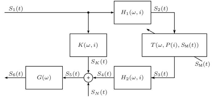
Fig. 6. Used signal model: Reader to reader channel  $K(\omega, i)$ , reader to tag channels  $H_1(\omega, i)$  and  $H_2(\omega, i)$ , tag reflection coefficient  $T(\omega, P, S_M)$ , reader input stage  $G(\omega)$ , modulation signal  $S_M(t)$ , carrier level signals  $S_1(t)$  through  $S_6(t)$ , noise  $S_N(t)$ ;  $i$  is the block index ( $\rightarrow$  block processing),  $\omega$  is the angular frequency,  $t$  is the time variable within one block
