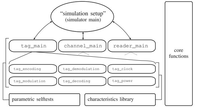
Fig. 2. Basic simulator structure: The complex bottom-level functions ( $reader\_*$ ,  $channel\_*$ ,  $tag\_*$ ) are handled by simple top-level interfaces ( $*\_main$ ); the user can construct the "simulation setup" in an interpreter fashion. All modules are verified by parametric selftests; core functions manage function/characteristic versions, logging and exceptions.
