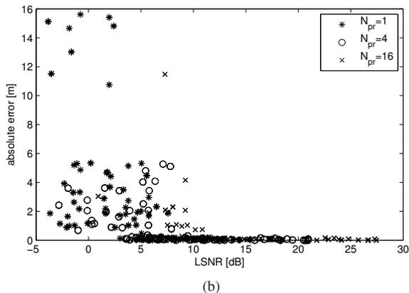
Fig. 3: Ranging results with a threshold  $c = 0.6$  for specific (a)  $E_p/N_0$  and (b) LSNR with respect to  $N_{pr}$  respectively.
