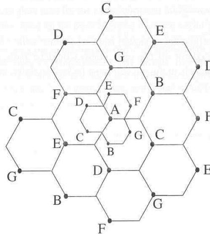
Figure 3.8 Illustration of cell splitting.
