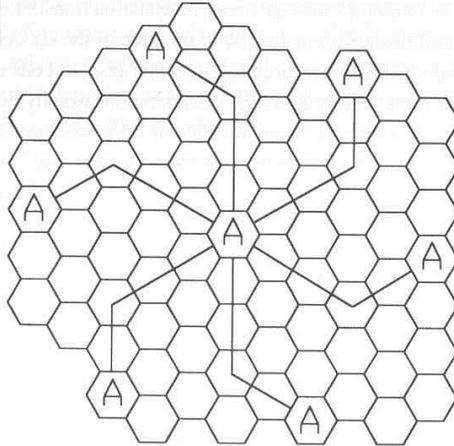
**Figure 3.2** Method of locating co-channel cells in a cellular system. In this example,  $N = 19$  (i.e.,  $i = 3$ ,  $j = 2$ ). (Adapted from [Oet83] © IEEE.)
