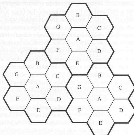
**Figure 3.1** Illustration of the cellular frequency reuse concept. Cells with the same letter use the same set of frequencies. A cell cluster is outlined in bold and replicated over the coverage area. In this example, the cluster size,  $N$ , is equal to seven, and the frequency reuse factor is  $1/7$  since each cell contains one-seventh of the total number of available channels.
