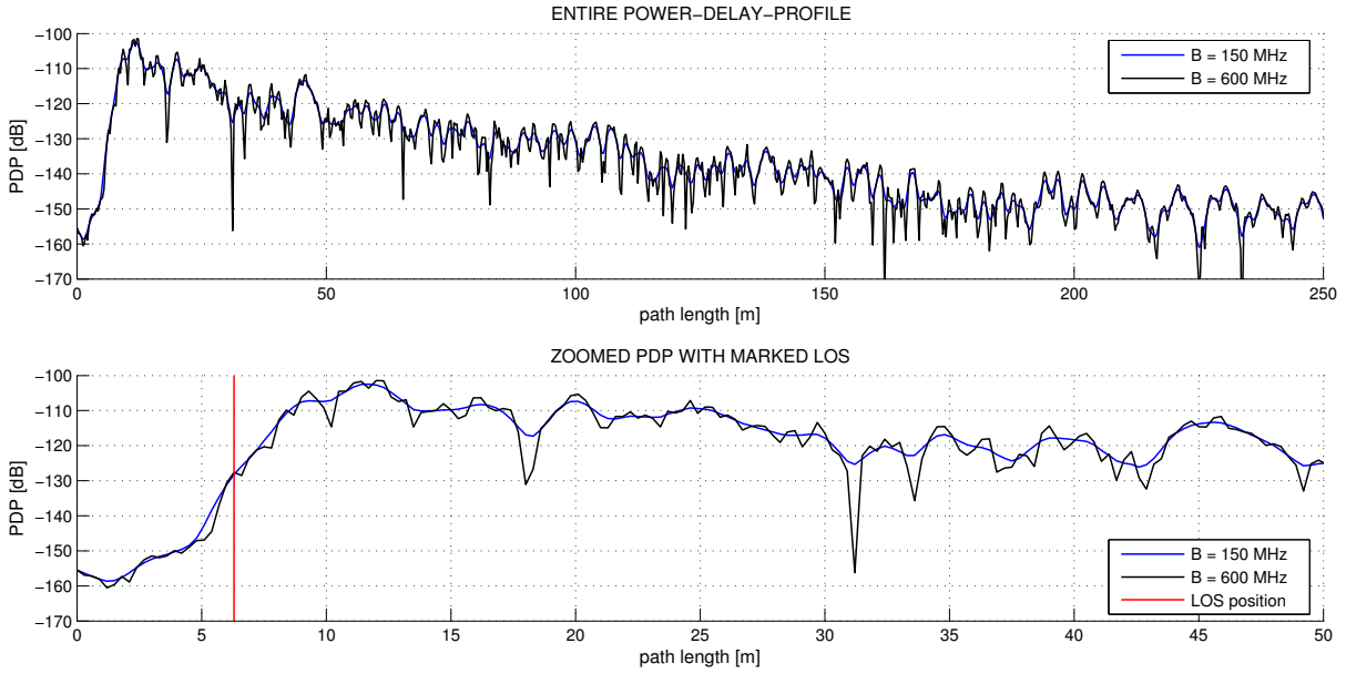
Figure 5.10: Hard-to-detect LOS (reflections close to an attenuated LOS plus strong gate reflections). Note that the LOS is no longer visible at B = 150 MHz.
